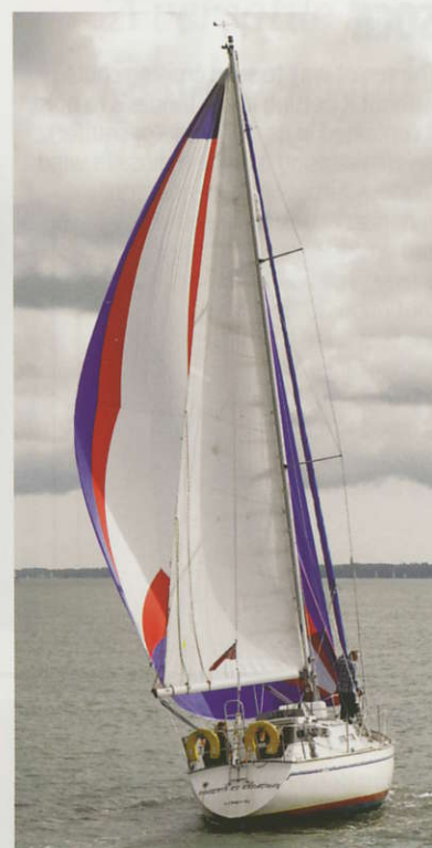
On the wind, tighten the halyard and tack strop for a straight leading edge
